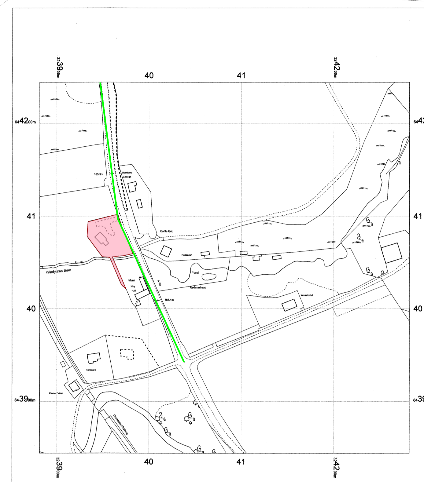
LOCATION PLAN -1:2500 with Visibility Splays of 2.4M x 160M
